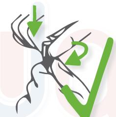
**Step 2:** Tweak and meanwhile press the cap to the tube.
